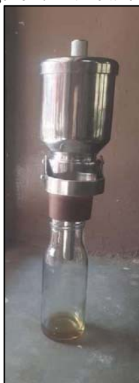
Figure 5: Filtration of artificial urine through filter funnel.
